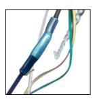
Heat-Shrunk Sealed, Concealed Wiring
